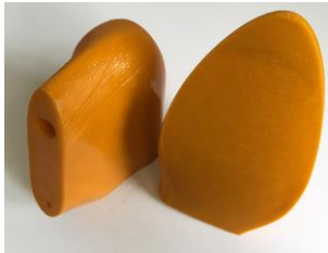
Fig. 6. An example of a 3D Printed Shoelast printed in two pieces [5]
